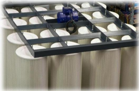
The Cartridge filters are tough spun bonded Polyester with a filtration capability below 1 Micron (1/1000<sup>th</sup> of a Millimeter!) to ensure a clean, safe working environment. They are encased in heavy perforated metal cylinders to maintain shape and prevent large waste particles entering the pleats. Durable and
