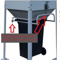
Clamping pressure is important to achieve an adequate seal
