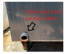
Drain plug if not sealed properly also causes liner rising, a bung should be fitted with a sealant
